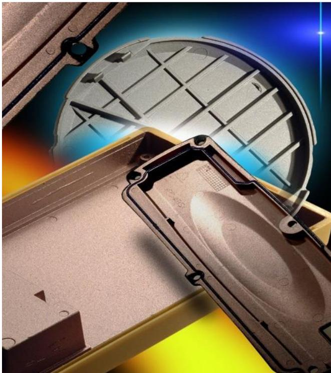
The most commonly used paints are conductive nickel, silver plated copper, or silver. Nickel paint is very common, but silver plated copper has become more attractive, particularly as it provides a better finish and performance. Applied at 25 micron thickness silver plated copper has no price premium over nickel.
